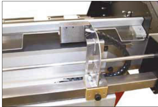
The optional side sensor will compensate for inaccurately wound rolls.
