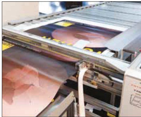
The table automatically aligns the media and feeds it into the cutter
