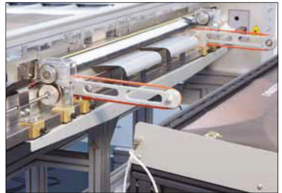
The exit sorting tools feeds the trimmed job to the collecting table
