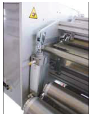
The pneumatic system makes roll loading easier
